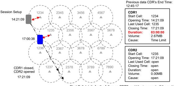
Start Cell details for the follow-on CDR2 could be inaccurate if the mobile device has moved since connecting with Cell ID 1235 at 17:00:38
