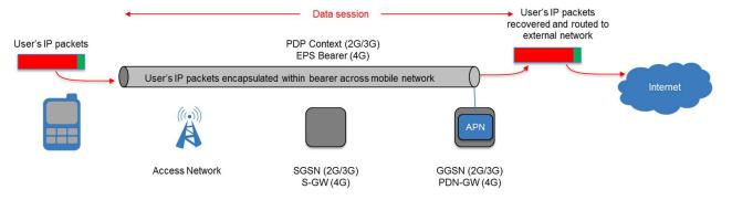
Access to a physical radio connection in a cell is provided to a mobile device, to carry data for a session, if it requests a connection. The physical connection is released if the network decides that is has been unused for too long – this access network 'idle timeout' usually takes place if the data connection has been idle for a relatively short time of between 10 seconds (in 4G/5G) to a few minutes (in 2G/3G).
